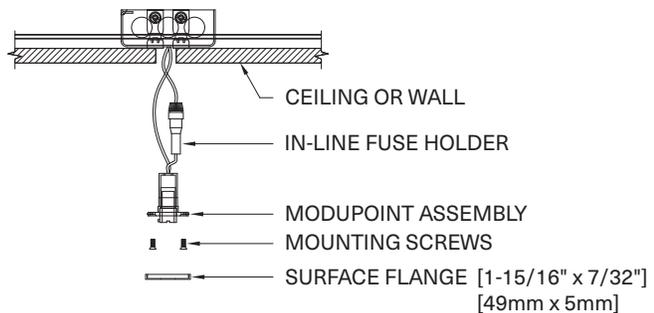
Housing: Recessed with 1-15/16" [49mm] surface flange
