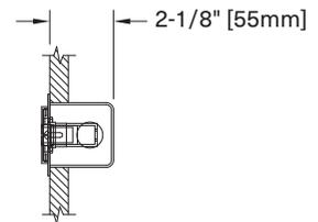
**Housing:** Recessed EQ Modupoint with 1-15/16" [49mm] surface flange is factory installed on plate
