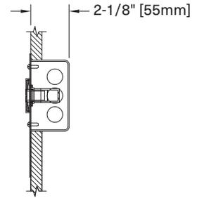
**Housing:** Recessed EQ Modupoint with 1-15/16" [49mm] surface flange is factory installed on plate
