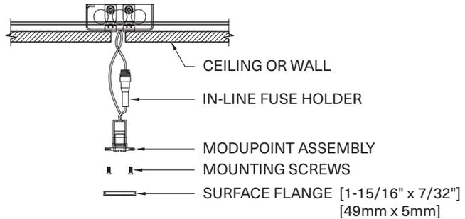
Housing: Recessed with 1-15/16" [49mm] surface flange
