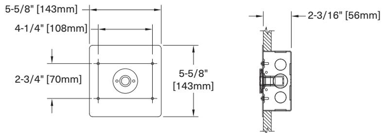
Housing: Recessed EQ Modupoint with 1-15/16" [49mm] surface flange is factory installed on plate
