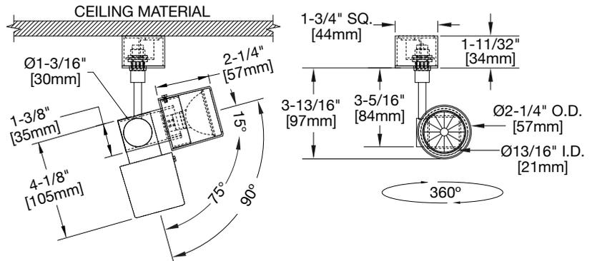
Housing: Fabricated aluminum and steel
