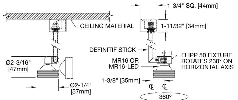
Housing: Fabricated aluminum and steel
